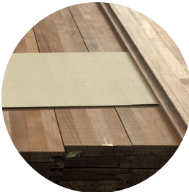
Band sawn face material and coated boards with – cardboard slip sheets between faces.
